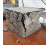
Fig 11: Specimen after failure in CTM
